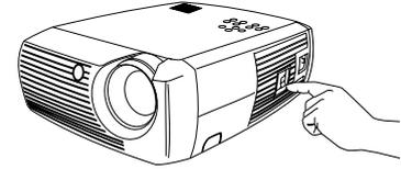
The LED flashes green and the fans start to run. When the lamp comes on, the start-up screen is displayed and the LED is steady green. It can take a minute for the image to achieve full brightness.
