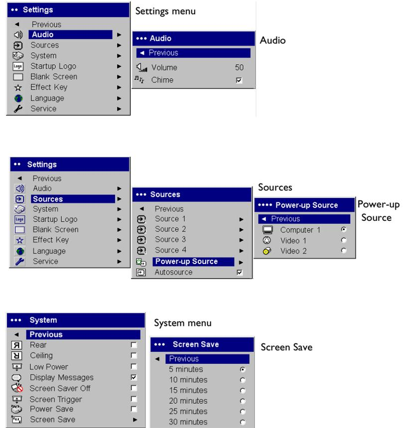
**Startup Logo:** allows you to display a blank screen instead of the default screen at startup, and when no source is detected.
